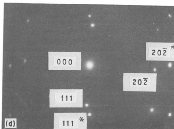
Figure 7 Comparison of populations A (left) and B (right). (a), (c) Transmission electron micrographs of lamellae; (b), (d) corresponding microdiffraction patterns with superimposed zone axis typical of relations A and B.
